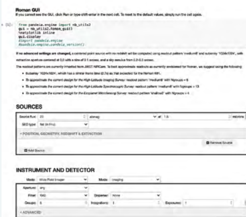
Pandeia provides a GUI as a Jupyter notebook for ease of use
