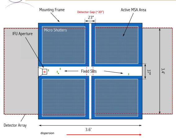
• The Micro-Shutter Assembly (MSA) is a 4 quadrant array of tiny configurable shutters. The entire array has nearly 250,000 shutters.
