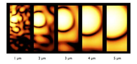
Slit throughput or slit loss is a function of wavelength and the relative placement of the science source in the MSA shutter
