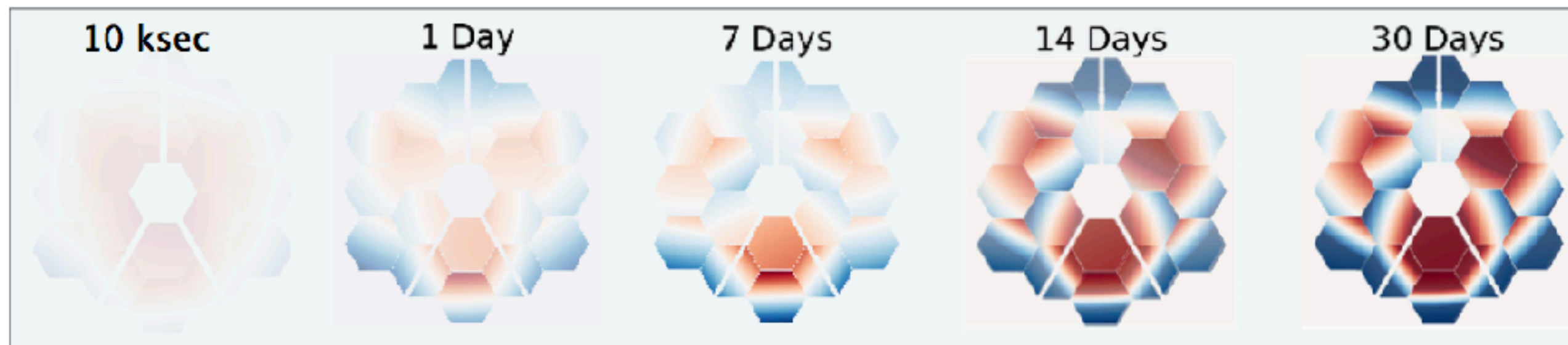
Model-predicted \Delta WFE from maximum hot-to-cold slew
