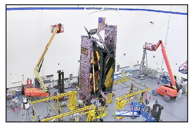
NASA's James Webb Space Telescope has been successfully folded and stowed into the same configuration it will have when loaded onto an Ariane 5 rocket for launch next year. (Credit: NASA, Northrop Grumman, May 14, 2020)
