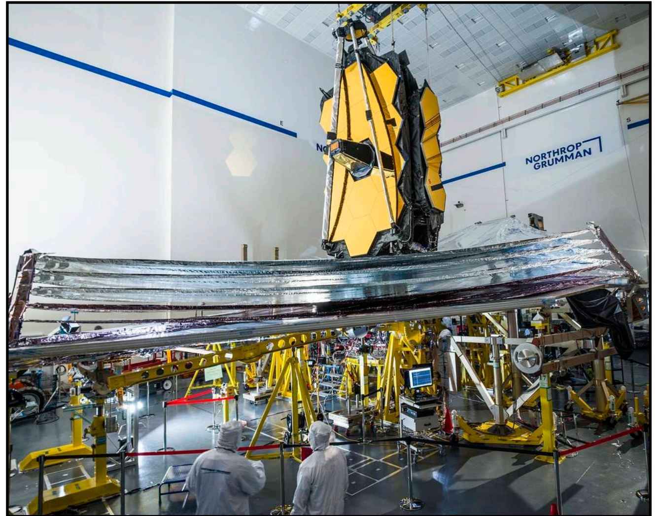
To help ensure success, technicians carefully inspect the James Webb Space Telescope's sunshield before deployment testing begins, while it is occurring, and perform a full post-test analysis to ensure the observatory is operating as planned. Credits: NASA/Chris Gunn
