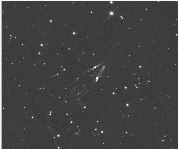
Example of a partially masked ghost which has imprinted onto an r-band stack (the field is ~10' across).
